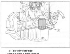
Remove with a filter wrench (Tighten with your hand)
